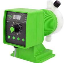
The AMSA digital series metering pumps feature smart microprocessor controls, providing outstanding accuracy with quartz timing. An LCD display is utilised for display of measured values, stroking rates, and assists with pump setup and calibration functions. A variety of input signals can be accepted depending on the model, see below. The AMSA series metering pumps have a self venting liquid end fitted. For medias that emit gasses, the self priming function ensures reliable metering.
