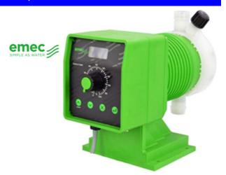
The AMS digital series metering pumps feature smart microprocessor controls, providing outstanding accuracy with quartz timing, and EEPROM storage of data and settings during power outages. An LCD display is utilised for display of measured values, stroking rates, and assists with pump setup and calibration functions. A variety of input signals can be accepted depending on the model, see below.
