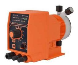
The KA series metering pumps have a self venting liquid end fitted. For medias that emit gasses, the self priming function ensures reliable metering.
